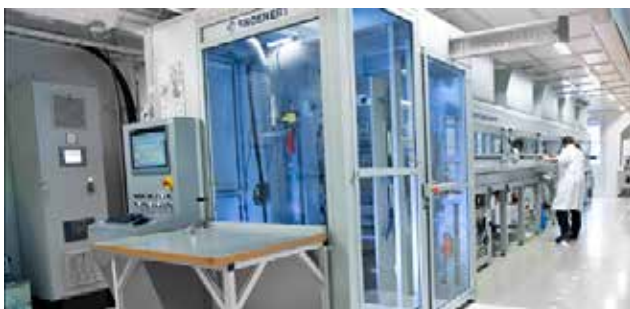
Fig 1 Thinfilm's R2R print line
