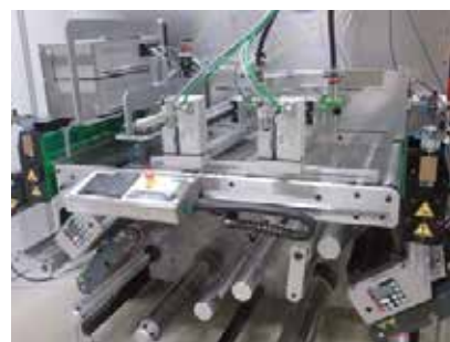
Fig 2 R2R step-and-go memory tester and programmer
